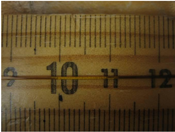
Figure 4.4. Photograph of Tenax microtrap packed in 530 \mu\text{m} i.d. fused silica tubing.
